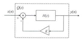
Find the system function of the closed-loop system, Q(z), and determine the values for the constant feedback gain K that result in a stable system. Assume that K is a real number.
